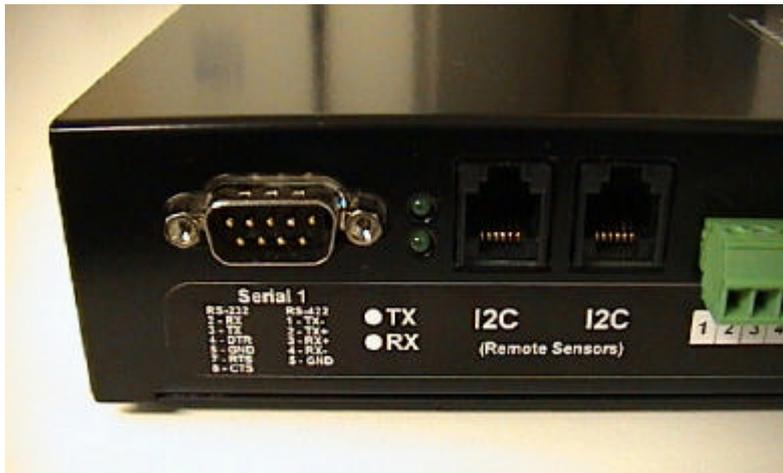
View of RS-232/RS-422 Serial and 2 x I2C ports
